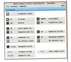
The RCP8 then forwards "BITE Packets" to the radar control workstation which is running the BITEX utility which provides a graphical user interface for monitoring of the system and for setting the IRIS alert status. An example of a BITEX maintenance screen is shown here for the transmitter.
